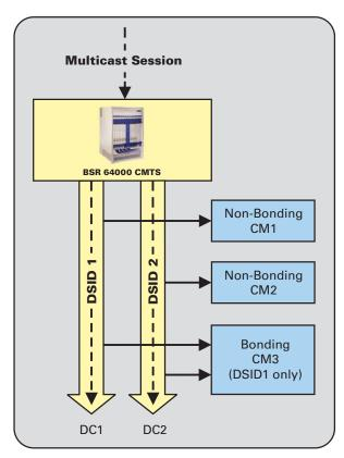
In this example, the CMTS is required to replicate the stream because there are both DOCSIS 3.0 and pre-DOCSIS 3.0 devices on the network that require the multicast stream. It is also possible in a mixed network for a multicast stream to be split over multiple downstream channels for bonding-capable modems, and then replicated on a single downstream for non-bonding capable modems.
