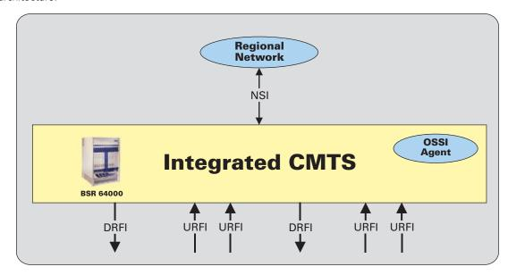
The I-CMTS is a single component/device that manages all aspects of the DOCSIS CMTS specification. Both the upstream and downstream channels are integrated into a single chassis.
