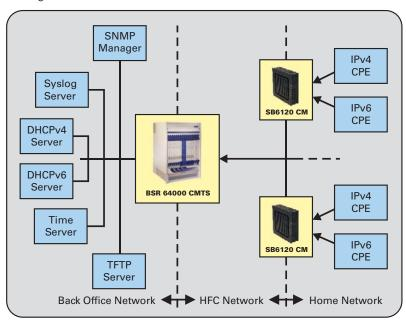
The above diagram illustrates a typical back office network configuration capable of supporting both IPv4 and IPv6.
